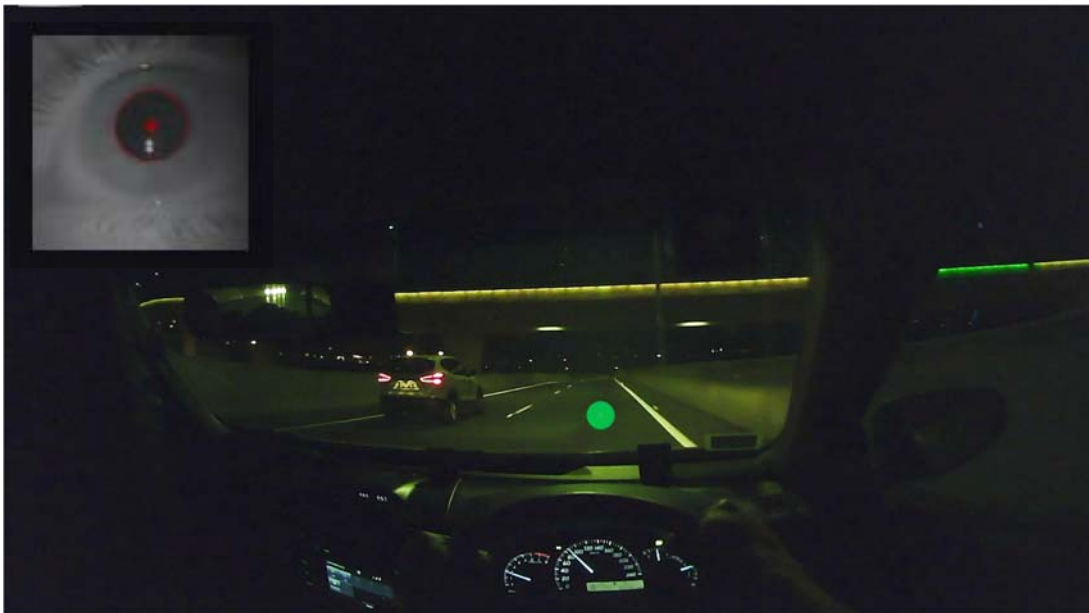
Figure 5-3: Screenshot of the eye tracking and pupil detection (upper left box)
