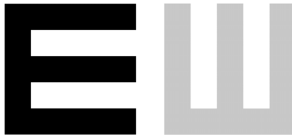
Figure 5-9: Schematic representation of the high 90% contrast (left) and low 22% contrast (right) tumbling E letters.
