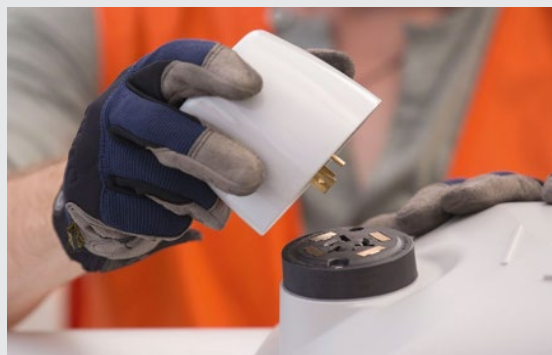
Figure 34 – A smart sensor light point controller plugs in to a luminaire mounted NEMA receptacle (Philips)
